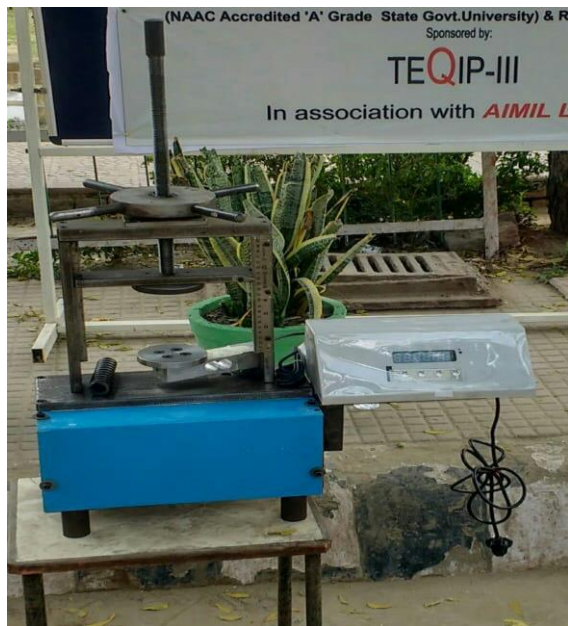
Figure 1: Spring load stiffness tester for helical springs
